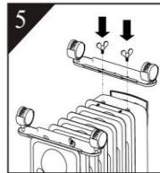
**IMPORTANT:** Please fit the wheel assemblies as per the diagram. Any other position may affect the stability of the heater.
